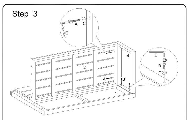
Attach seat frame (2) to left leg (4) using long bolts (A) and washers (C). Attach left leg (4) to back frame (1) using short bolts (B) and washers (C). Tighten all bolts with wrench (E). Hands tighten all bolts only and not tighten completely.
