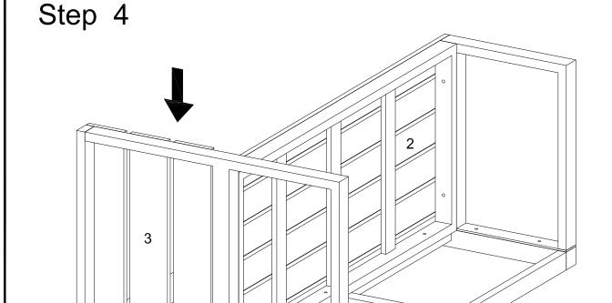
Attach right leg (3) to back frame (1) using bolts as guides.
