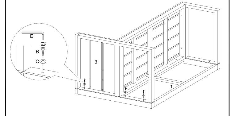
Attach right leg (3) to back frame (1) using short bolts (B) and washers (C) . Tighten short bolts (B) with wrench (E). Hands tighten all bolts only and not tighten completely.
