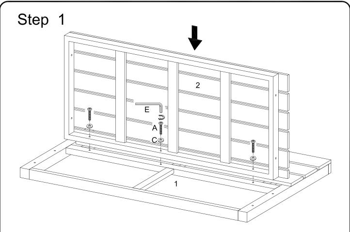
Attach seat frame (2) to back frame (1) using long bolts (A) and washers (C) . Tighten long bolts (A) with wrench (E). Hands tighten all bolts only and not tighten completely.
