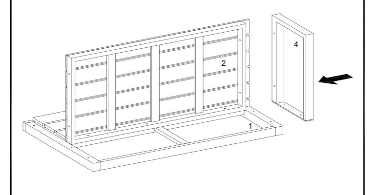
Attach left leg (4) to seat frame (2) using bolts as guides.
