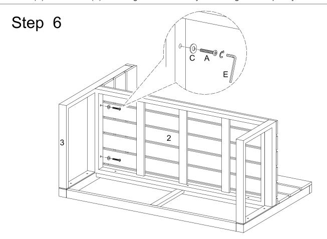
Attach seat frame (2) to right leg (3) using long bolts (A) and washers (C) . Tighten long bolts (A) with wrench (E). Hands tighten all bolts only and not tighten completely.
